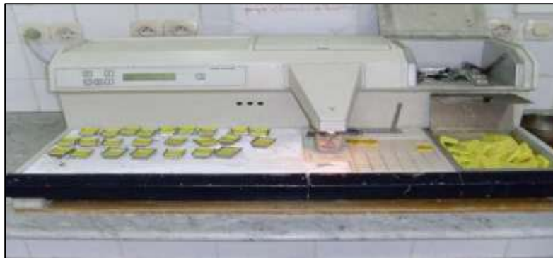
Figure.25: Complete embedding module.
